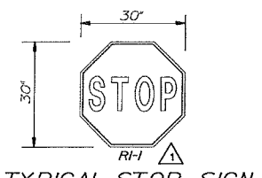
TYPICAL STOP SIGN (UNLESS OTHERWISE SPECIFIED)
