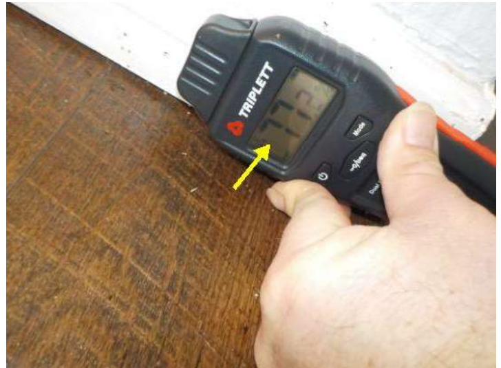
Advise several living room and kitchen walls are 66%-99% wet in numerous areas. Recommend having dehumidifiers placed in unit until moisture intrusion can be controlled.
