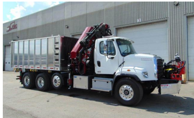
NEW BIK TREE-CARE SERIES TC-98/104 NEW FREIGHTLINER 108SD 4-AXLE NEW 16' ALUM DUMP AND SG-280 SAW
