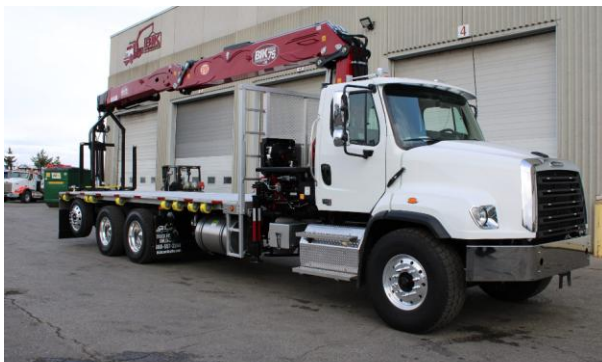
NEW BIK WALLBOARD CRANE SERIES WC-75 BY PM FREIGHTLINER 114SD 3-AXLE DIESEL TRUCK 500 HP, CUMMINS DIESEL, AUTOMATED 18SPD TRANS
