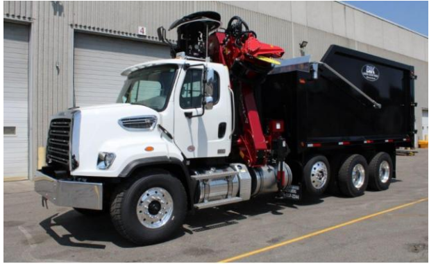
BIK DEBRIS CRANE SERIES Z-BOOM DC-18Z FOLDABLE WITH GRAPPLE ON FLINER 108SD 4-AXLE & 18' DUMP BODY
