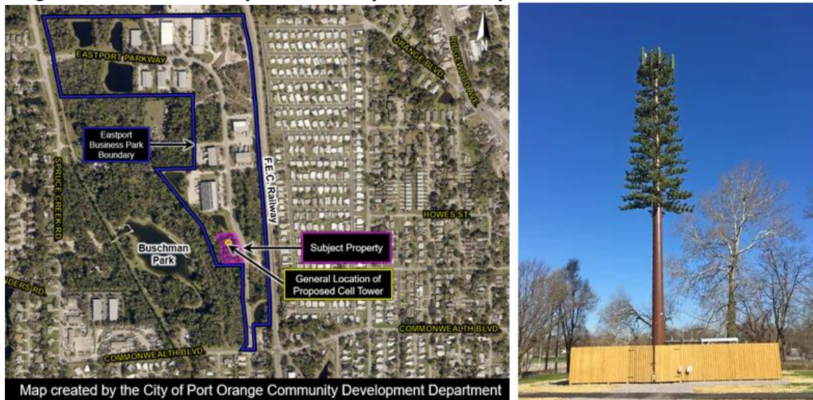
Figure 1. Location Map and Example of Monopine Communications Tower
