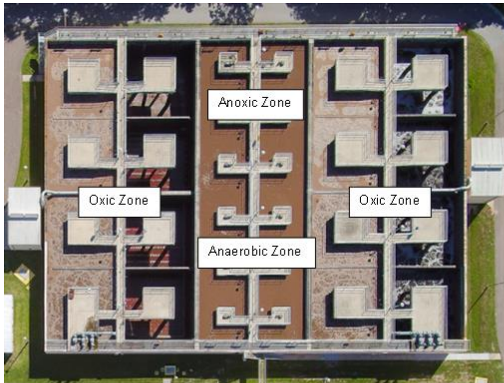
FIGURE 12: A 2 O TREATMENT STRUCTURE
