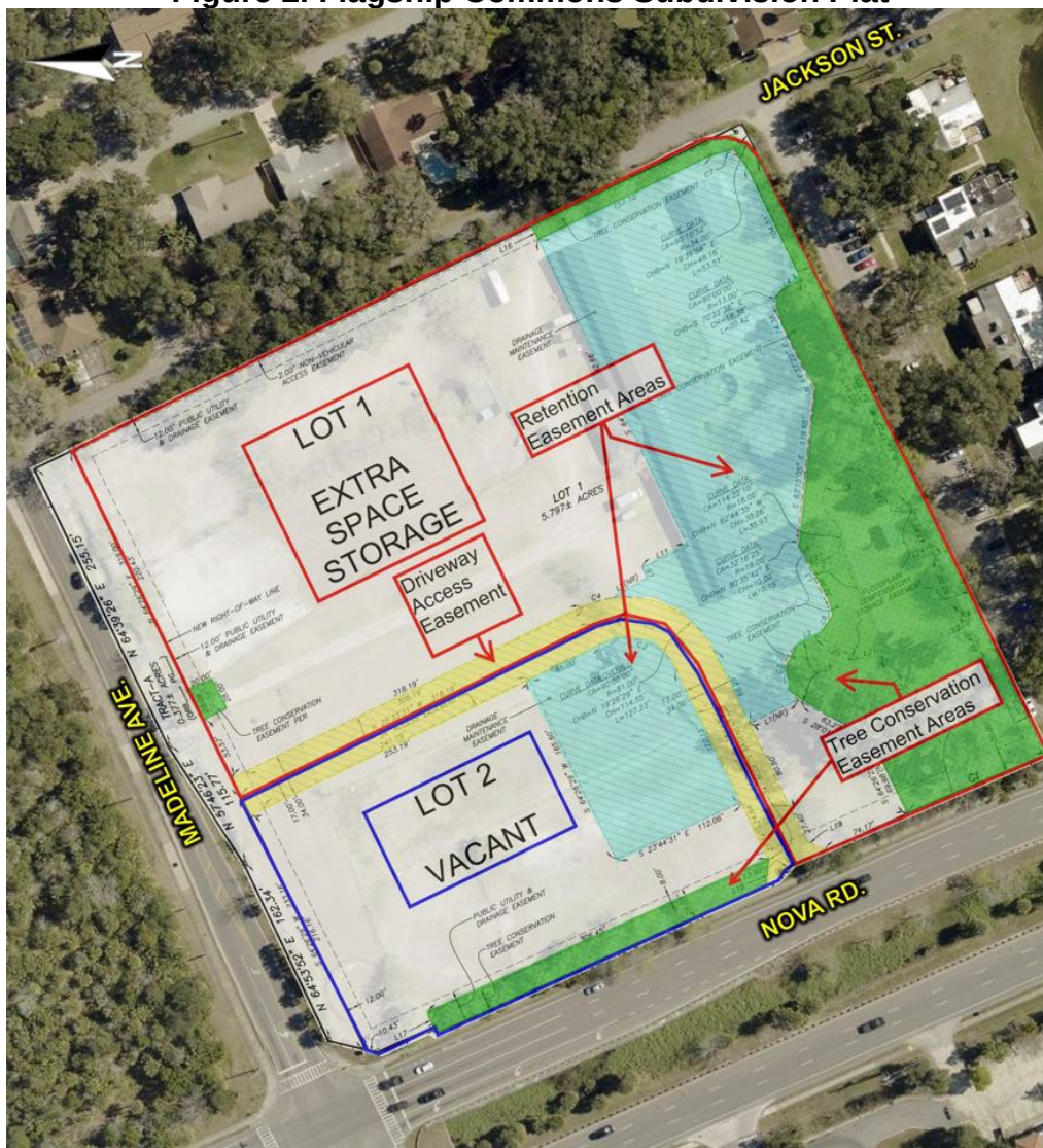
Figure 2. Flagship Commons Subdivision Plat
