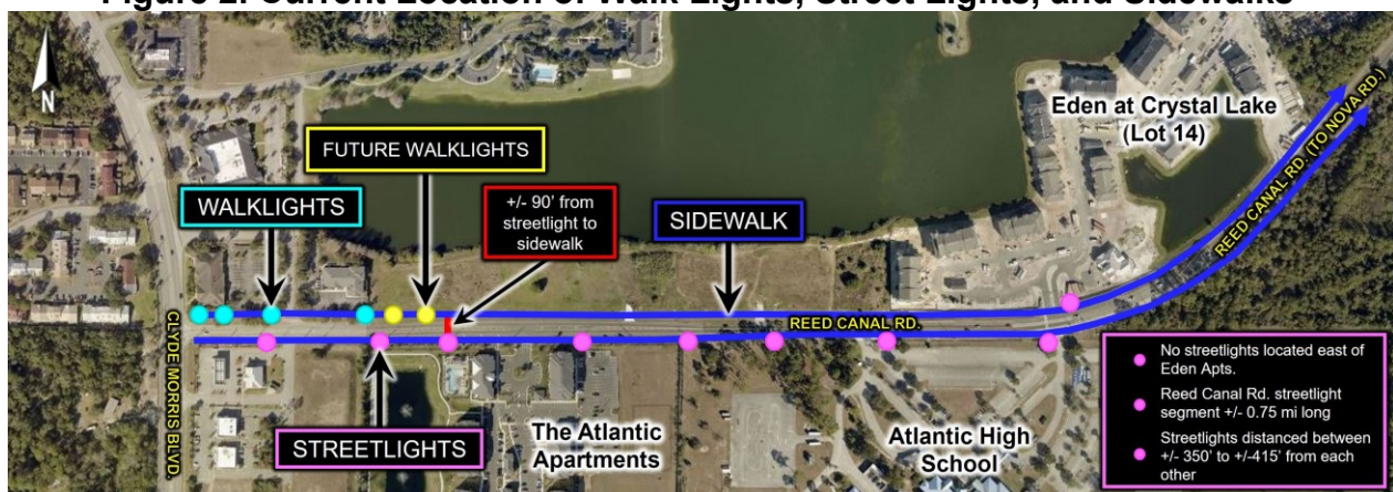
Figure 2. Current Location of Walk Lights, Street Lights, and Sidewalks
