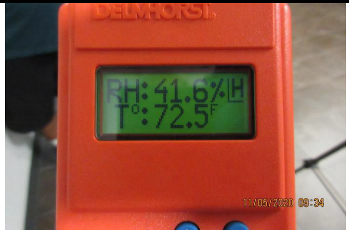
Photograph 14 1st Floor East Corridor Temp 72.5° / Relative Humidity 41.6%
