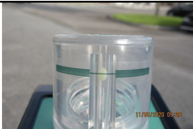
Photograph 63 Pump Calibrated to 15 Liters
