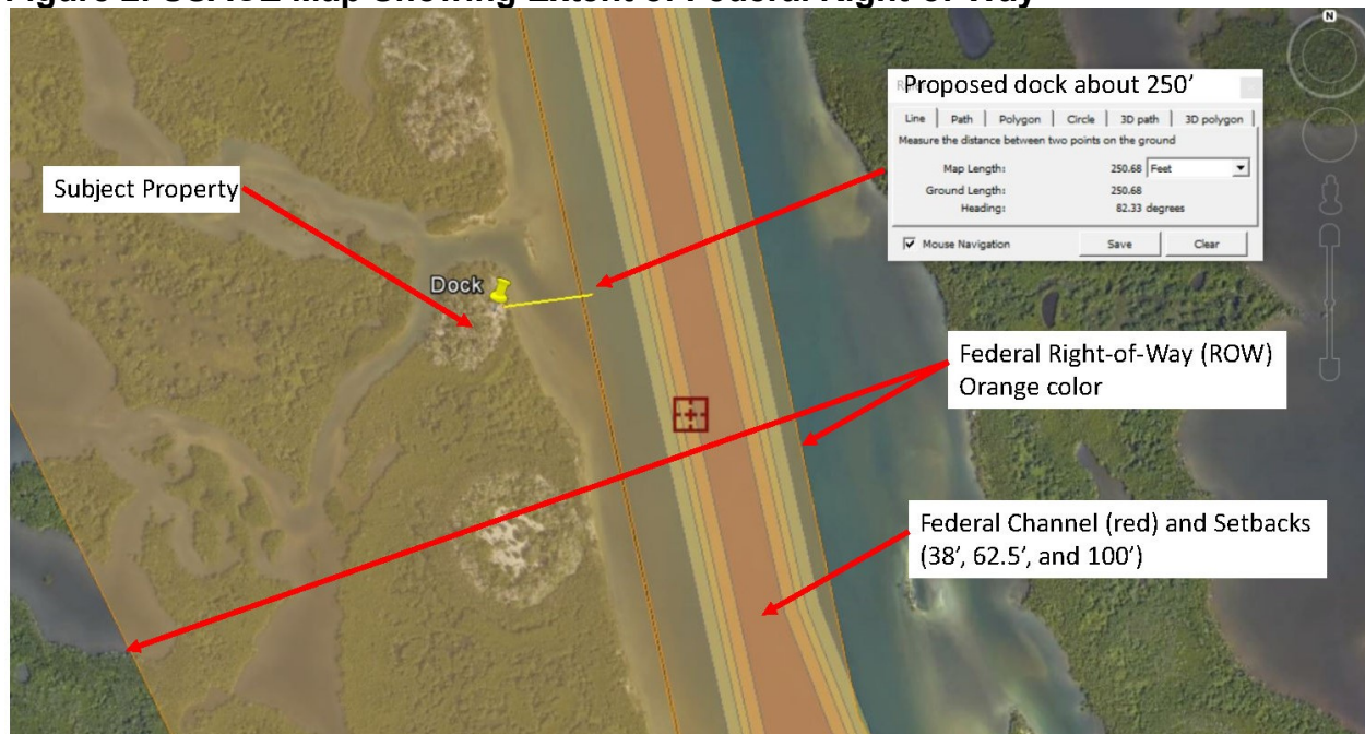
Figure 2. USACE Map Showing Extent of Federal Right-of-Way
