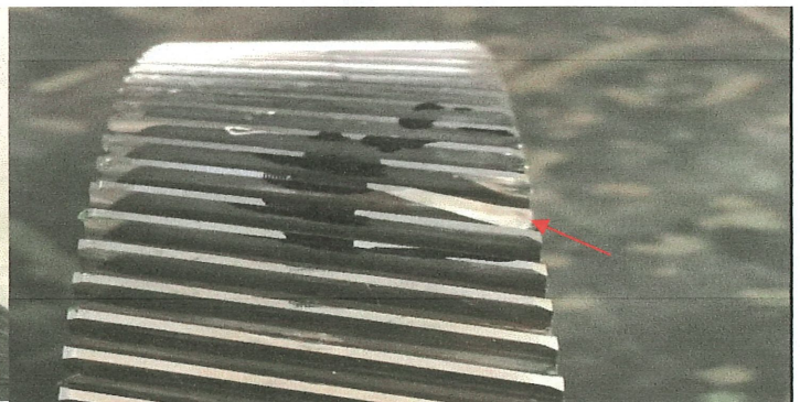
Broken tooth on change gear
