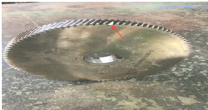
Broken tooth on change gear
