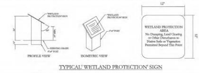
TYPICAL WETLAND PROTECTION SIGN
